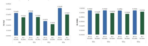
As can be concluded, with the digitalization of the water distribution and with the help of advanced analytical solutions, it was possible to reduce costs by 21%.
